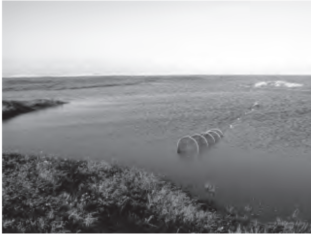
FIGURE 60 Fyke net deployed in a river. A Fyke net consists of two single-mouth hoop traps set on either end of a lead. The traps may be baited to attract certain species of turtles. Other species that are not attracted to bait follow the lead into the traps. (Photo courtesy of Alexandre M. Batistella.)
