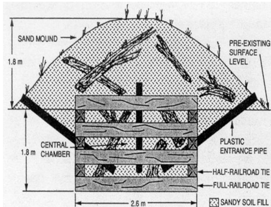
Figure 14. Side view of underground hibernation chamber for snakes and other wildlife. This drawing shows the method of construction using 18 pressure treated railroad ties and 10 cm diameter PVC pipes (Zappalorti and H. Reinert, Herpetological Associates, Inc).
